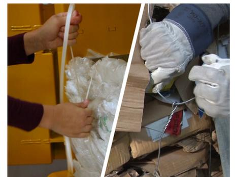
You can use either plastic strapping or steel wires to tie the finished bales.
