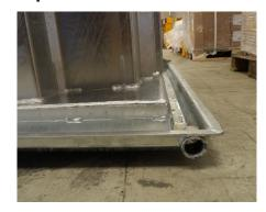
A draining system leads liquids out of your baler during compaction of wet waste.
