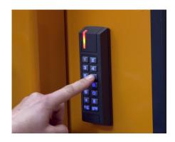
A digital auto lock enables baler loading but restricts access to run a press cycle.
